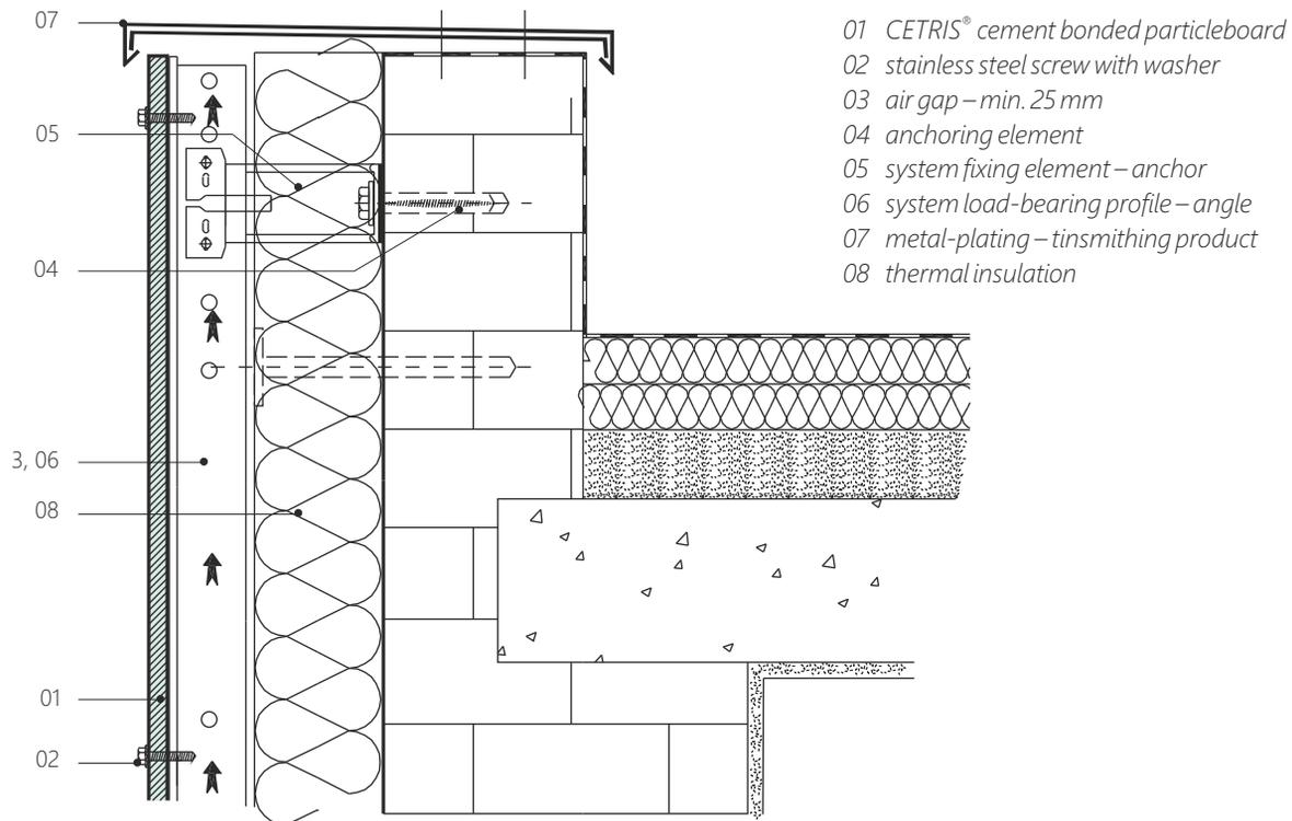
Detail of bottom ending with overlap. CETRIS® board on system profiles, VARIO system
