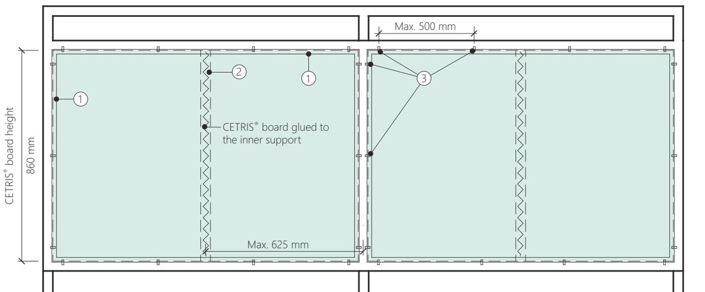
When using a CETRIS® board of thickness 10 mm, the maximum possible spacing of the inner vertical reinforcements is 420 mm. A suitable type of the peripheral lath is the F profile PROAL 74008.
