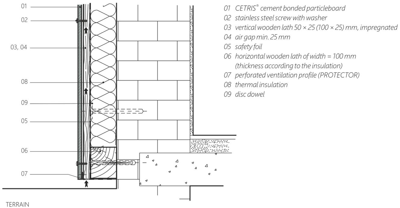
**Detail of bottom lining with sheet metal lining - CETRIS® board on wooden grid, VARIO system**
