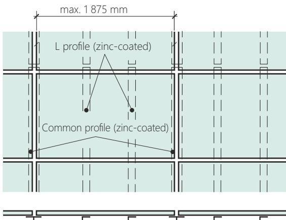
**Dilatation – grid of aluminium or zinc-coated profiles**
