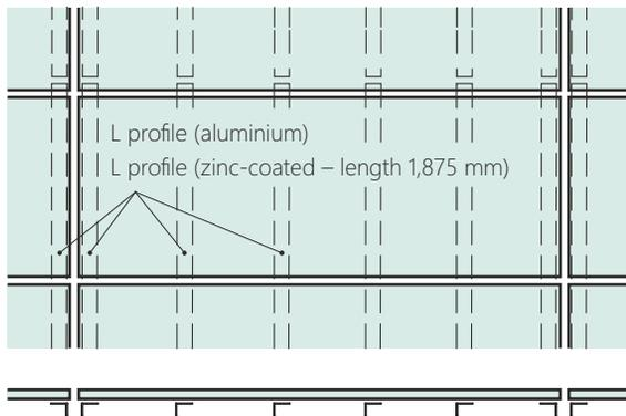
For façades wider than 8 metres, it is necessary to ensure continuous vertical dilatation in the load-bearing construction – i.e. the base construction at the points of the vertical joint must be resolved using two separate profiles.
