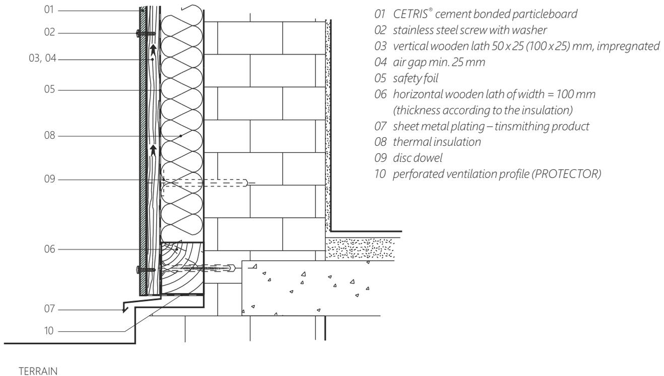
Detail of upper lining with roof construction overlap. CETRIS® board on wooden grid, VARIO system
