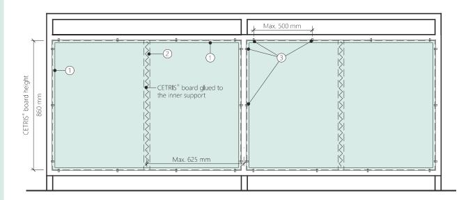
When using a CETRIS® board of thickness 10 mm, the maximum possible spacing of the inner vertical reinforcements is 420 mm. A suitable type of the peripheral lath is the F profile PROAL 74008.
