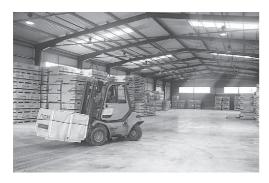
CETRIS® cement bonded particleboards are stored on wooden pallets allowing for forklift handling. The boards are fixed to the pallet by crosswise tying of the boards to the pallet. Lengthwise tying on customer request only.
