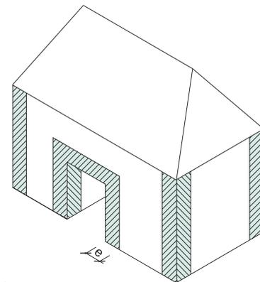
Exposed positions on building edges, openings, passages and thoroughfares in the buildings.
