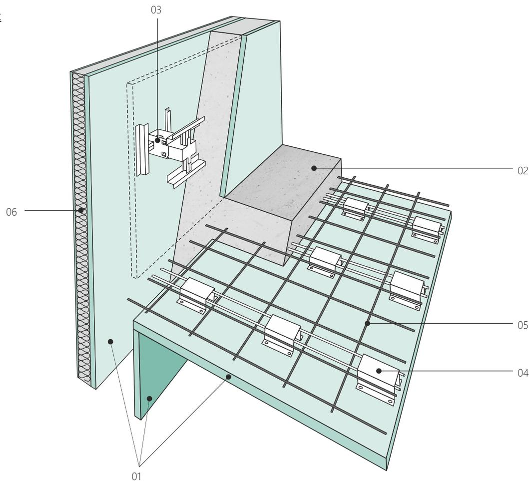
01 CETRIS® BASIC cement bonded particleboard, thickness 24 mm)
