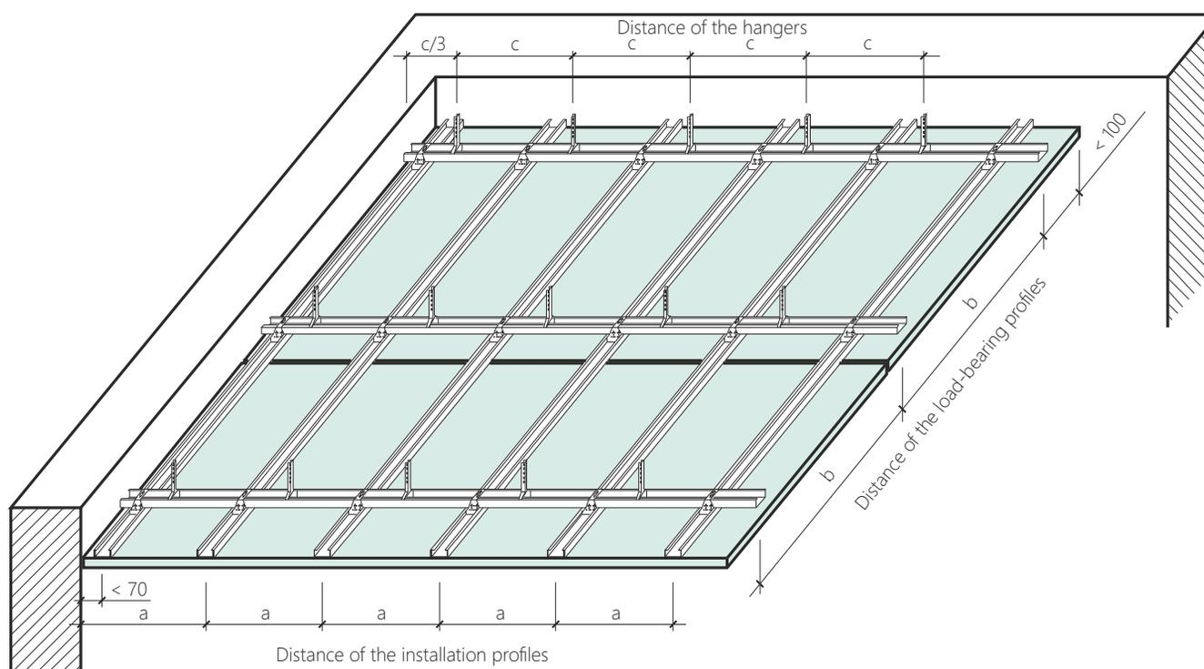
Fig. 2) Schematic drawing of the load-bearing construction of the ceiling for cladding with CETRIS® cement bonded particleboard (thickness 2 × 12 mm)
