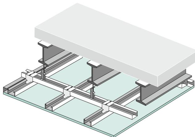
**Fire resistance of the ceiling construction protected by a horizontal membrane – hanging ceiling of composition CETRIS® BASIC 12 mm:**
