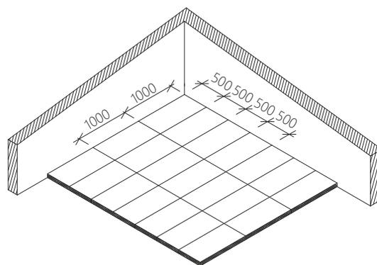
7 – A dilatation joints with a width of 15 mm is created around the vertical constructions (walls, pillars etc.). It is recommended to place a 15 mm wide mineral wool or polystyrene strip into the dilatation joints along the vertical constructions to prevent clogging of the dilatation joint during subsequent work. This tape is cut to the desired height upon completion of the final surface finishing of the floating floor before installation of the floorings.
