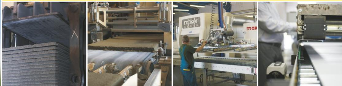
**CETRIS® cement bonded particleboards** are produced by pressing a mixture of wooden particles and portland cement with water. The surface is smooth, the color is cement-like grey.
