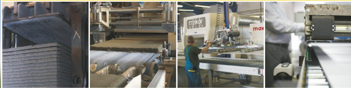
CETRIS® cement bonded particleboards are produced by pressing a mixture of wooden particles and portland cement with water. The surface is smooth, the color is cement-like grey.
